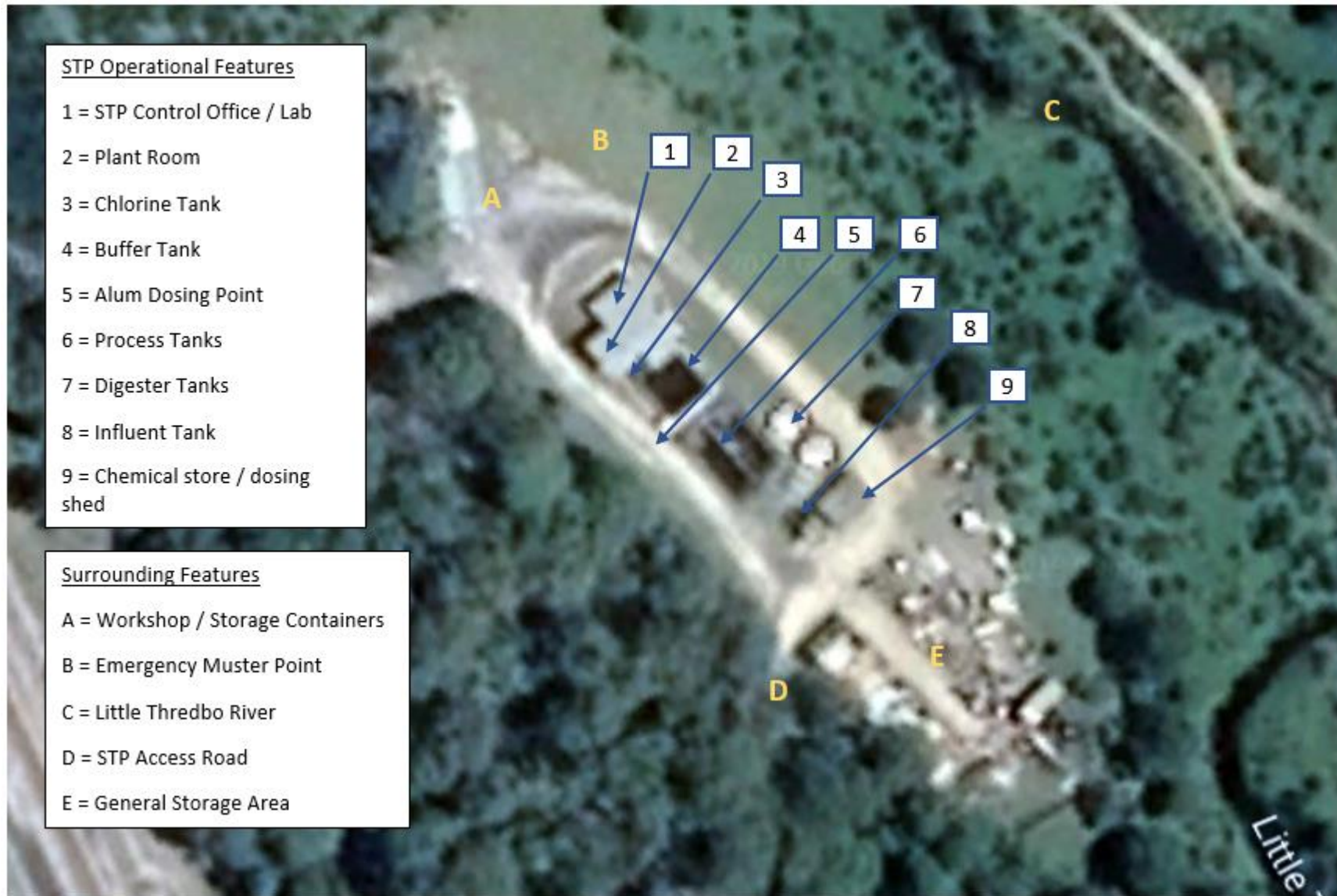
Figure 9.3 STP Operational Features
